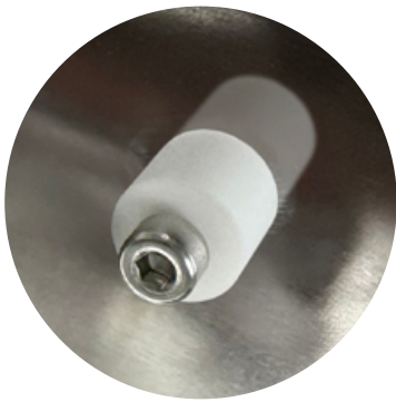
Electrode located on the inner wall of the sterilization chamber, just above the water coil.
